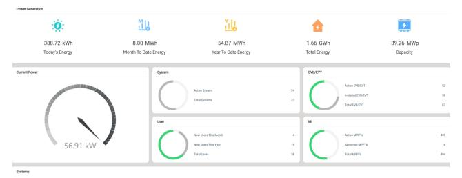
Today's Energy: the total energy harvest of all microinverters on the current day under the distributor account. Month To Date Energy: the total energy harvest of all microinverters in the current month under the distributor account. Year To Date Energy: the total energy harvest of all microinverters in the current year under the distributor account.
