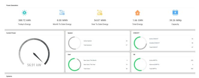
**Current Power:** the total generated power of all microinverters on the current day under the distributor account by the time the account is logged in to.
